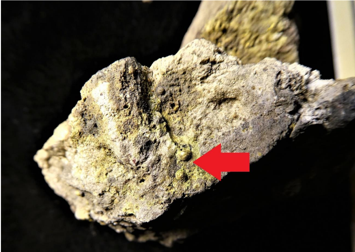
Figure 7. Another Vindicator mine gold ore specimen that William Hosley collected and roasted. Note the gold bubbles indicated by the red arrow on the surface of the rock. Field of view is 2.5 cm. From the private collection of Kathleen Liddy. Photo date 2021 by S. W. Veatch.
